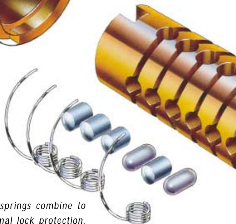
*Side pins and springs combine to provide additional lock protection. Undersized or incorrectly formed keys will activate traps for added security.*
